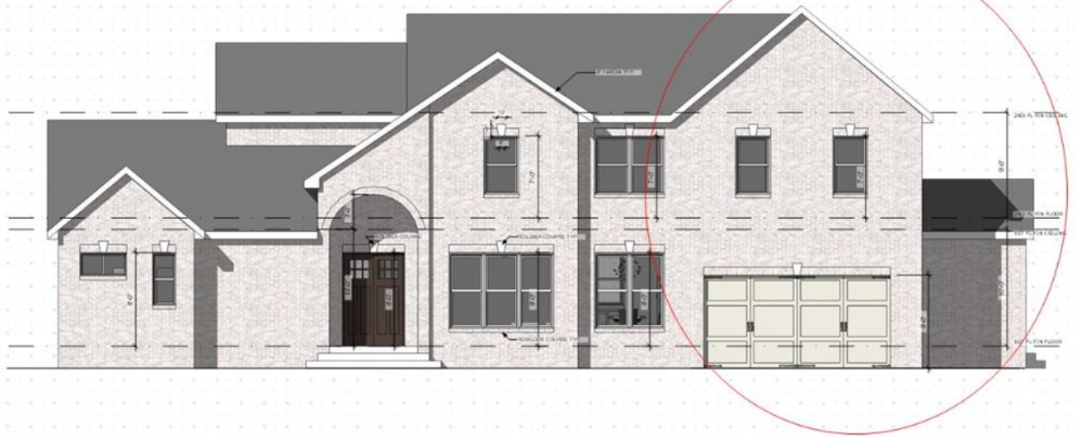
FRONT ELEVATION 1/4" = 1'-0" NOTE: ALL SIDES BRICK
